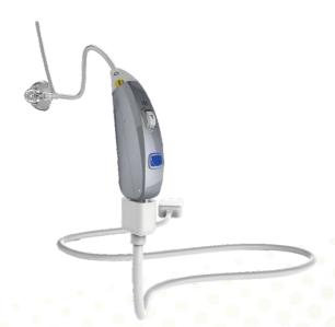
Consumers will appreciate the universal MICRO-USB interface and an unprecedented charge time of less than 2 hours for an average 20 hours of use-time. The break-through intelligent charging chip circuit minimizes heat and makes 'green' technology a practical really for hearing aid users.
